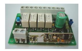
The decoder board HCS-DEC-1-2-4/F is a 1-2-4 channels central unit which can be matched with any HCS Keeloq encoded keyfob programmed with Aurel manufacturer code.
